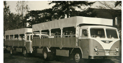
Underfloor vehicle modified into two-floor vehicle, a first in Japan Mammoths carrying 28 Honda Dreams
